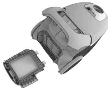
7. If the **filter lid comes loose**, restore by positioning the two hinges at the bottom and push the filter lid back until both of the two buttons click in.
